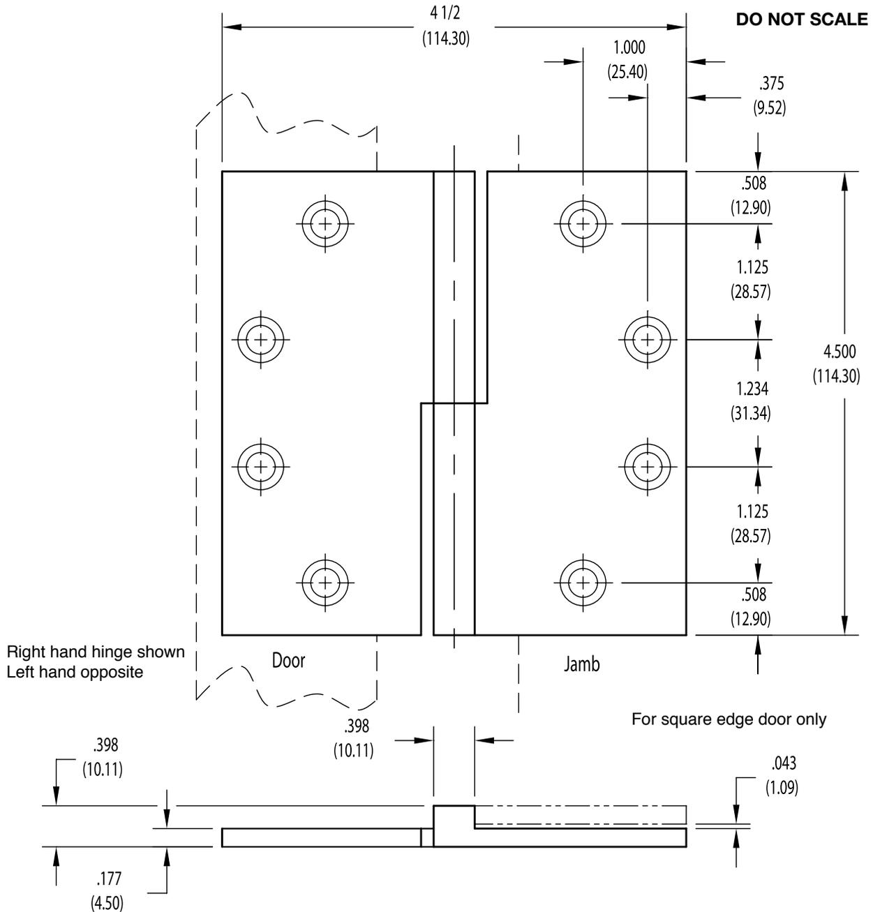
McKINNEY Square Barrel Hinges are made in size, gauge and with screw holes located to conform to this drawing.
