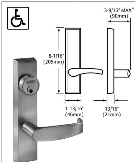
The 700 Series ET Control is sold separately from the exit device and can be used with 8888 & 8810 Exit Device. The trim is non handed and is through-bolted to the chassis for greater security and durability. Available in 7 functions and SARGENT Studio, Coastal and standard lever designs to accommodate most requirements.
