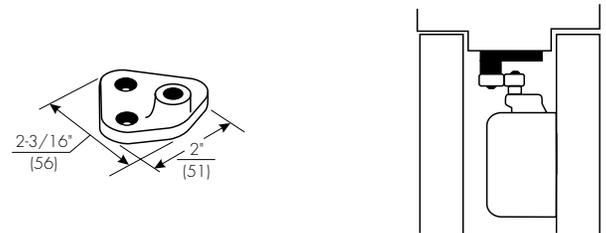
**Mounting between Doors - #2018 Soffit Bracket:** For use where insufficient space between companion doors does not permit use of other soffit plates. This bracket permits mounting of the closer between doors with as little as 3" (76mm) of header space. Permits closer arm to clear up to 5/8" (16mm) high stop.
