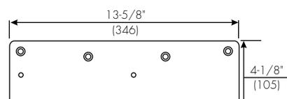
**Narrow Frame - #7786 Back Plate:** For use where a narrow frame face prevents the closer from being mounted directly to the frame. This back plate must be used for closer mounted on a frame between 1-7/8" and 3-1/8" (48 and 79mm) in height.
