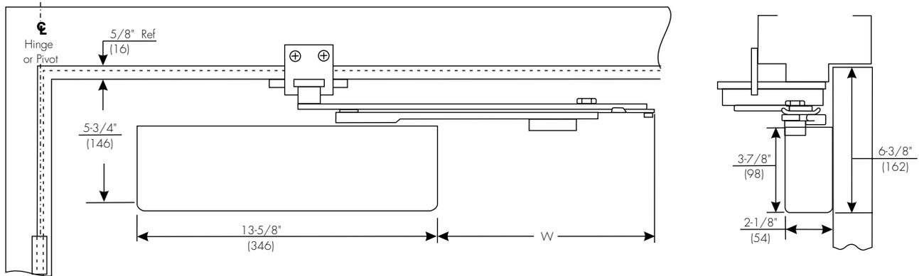
Mounting holes for closer body are spaced 2-3/8" (86mm) vertically x 6-3/4" (171mm) horizontally.
