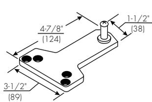
**Standard Installation - #1618 Soffit Plate:** Supplied standard with parallel arm closers. It can be mounted where the frame soffit is as narrow as 1" (25mm). Specify **1618A-SS** for stainless steel soffit plate.
