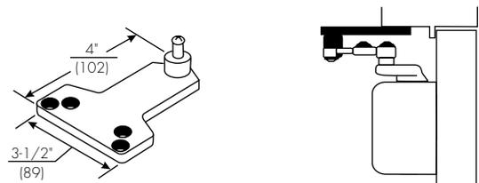
**Blade/Applied Stop - #2018D Soffit Plate:** For use where a blade or applied stop does not permit installation of the standard soffit plate. Mounts to either the frame soffit or rabbet. Since this soffit plate projects 7/8" (22mm) less than a standard soffit plate, it requires a minimum frame reveal of 1-1/2" (38mm). Permits closer to clear up to a 5/8" (16mm) stop.
