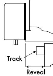
**Slide Track - #7786JP Back Plate:** Required for frames with standard 2" (51mm) profile face. Without plate, minimum 4" (102mm) face frame required.
