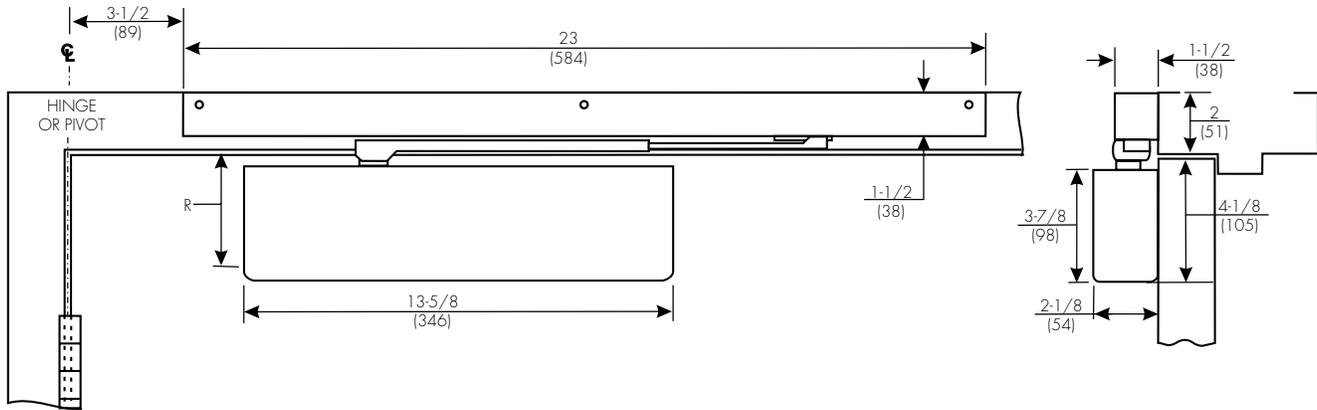
Mounting holes for closer body are spaced 2-3/8" (86mm) vertically x 6-3/4" (171 mm) horizontally.
