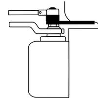
**Molded/Bull Nose Trim - #2403-3/4 Bracket:** This bracket is similar to - but longer than - the 2403B bracket. It is designed to accommodate frame rabbets from 2" to 2-7/8" (51 to 73mm) deep.
