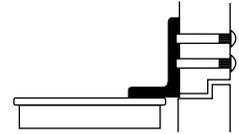
**Additional Support - #6190 Reinforcing Bracket:** Standard for use with all Parallel Arm *Unitrol* Door Controls. Provides additional support to the soffit plate on installations with door frame reveals from 1-7/8" to 4-5/8" (48 to 117mm).
