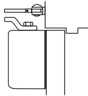
**Narrow Top Rail - #7786 Drop Plate:** For use where the narrow top rail of the door prevents the closer from being mounted directly to the door surface. This drop plate must be used for closer mounted on a top rail between 1-7/8" and 3-3/8" (48 and 86mm) in height.
