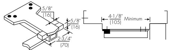
**Wide Frame - #6191 Reinforcing Kit:** Optional for use with all Parallel Arm *Unitrol* Door Controls. Used to support the soffit plate on installations with wide frames. Clamps may be used with or without the spacer block, depending on frame conditions.
