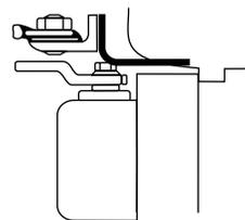
**Molded/Bull Nose Trim - #80 Bracket:** For use where the door frame has molded or bull nose trim which will not accept a standard hold open shoe. It is mortised into the frame rabbet, and projects beyond the face of the frame. It will accommodate a rabbet up to 2" (51 mm) deep. This bracket is used in combination with the standard hold open mounting shoe.
