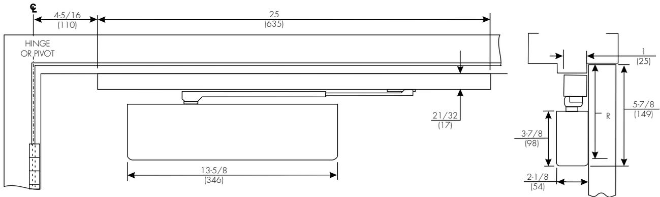
Mounting holes for closer body are spaced 2-3/8" (60mm) vertically x 6-3/4" (171mm) horizontally.
