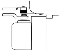
**Molded/Bull Nose Trim - #2403B Bracket:** For use where the door frame has molded or bull nose trim which will not accept a standard non-hold open shoe. The bracket is mortised into the frame rabbet, and projects beyond the face of the frame. It will accommodate a frame rabbet up to 2" (51 mm) deep.
