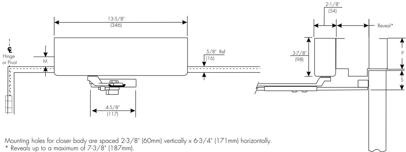
Mounting holes for closer body are spaced 2-3/8" (60mm) vertically x 6-3/4" (171mm) horizontally.
