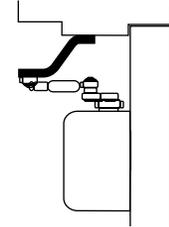
**Flush Transom - #2022 Angle Bracket:** For use where rabbeted or flush transom conditions prevent installation of a soffit plate. Used in combination with the 1618 soffit plate, or may be used in combination with the 2018S soffit plate when it is necessary for the closer arm to clear a separate overhead door holder.
