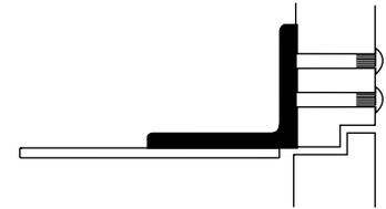
**Flush Rabbeted Transom - #2019L Angle Bracket:** For use where flush transom conditions prevent mounting of the standard soffit plate. This bracket is used in combination with the standard soffit plate.
