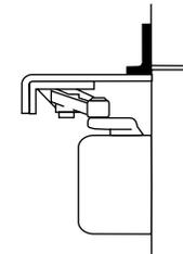
**Parallel Hold-Open - #1628H Adapter Plate:** Supplied standard with all parallel arm hold-open closers. It can also be used to convert regular arm or top jamb hold-open arms to parallel arm installation. It can be mounted where the frame soffit is as narrow as 1" (25mm).
