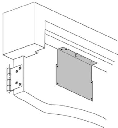
Metal templates help the installer locate the correct mounting holes for several parallel arm applications.
