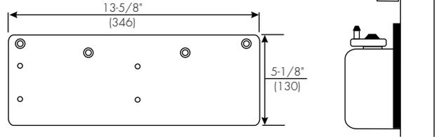
Soffit Plate Reinforcing Brackets (for Parallel Arm)
