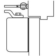
**Overhead Door Holder - #7786OH Drop Plate:** For use where a surface or concealed overhead door holder prevents normal arm mounting screws to clear the bottom of the door holder. This places the centerline of the arm mounting screws at 2-7/8" (73mm) from the top of the door.
