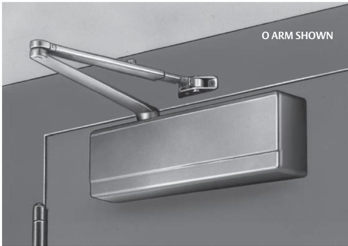
The standard application of the 1431 door closer is the most common and the most desirable. The closer mounts on the hinge (pull) side of door (except when the W Corner Bracket is used). Note: This application is not recommended on exterior doors swinging out, since the closer is not protected from weather. The cover projection normally limits the door opening to a maximum of 160°.
