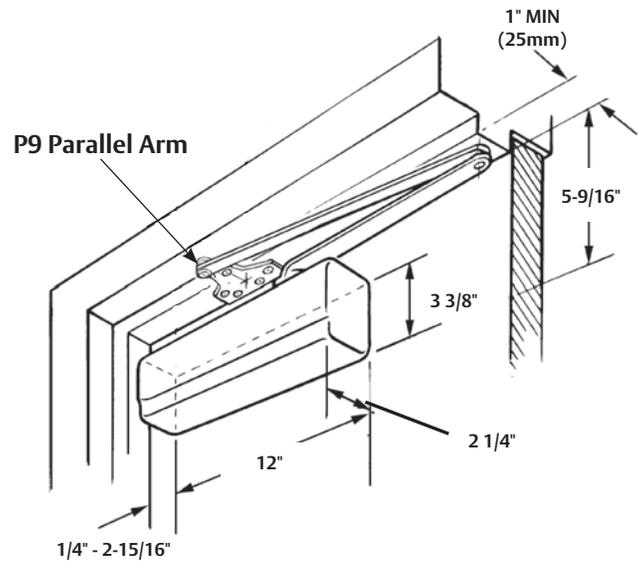
Parallel Arm Applications - The 1431 closer is mounted on the push side of the door with the arm under the frame parallel to the face of the door. This application is well suited for narrow face frames and deep reveal applications. The closer arm does not project into the room, and the door can be swung open much farther than in Top Jamb Application.
