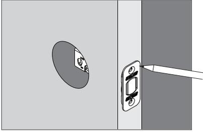
5b Remove bolt and drill two 1/8" pilot holes.
