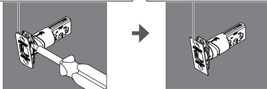
1c Install the bolt into the door.
