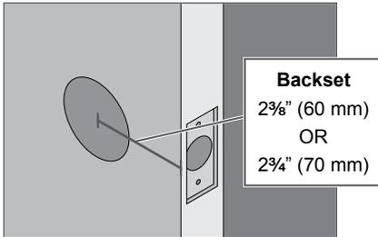
If the measurement is 2 3/4" (70 mm), extend the bolt.
