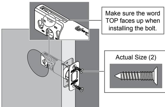
1d Install the strike into the frame.
