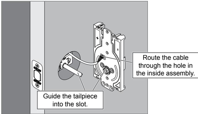
3c Secure the inside assembly with two screws.
