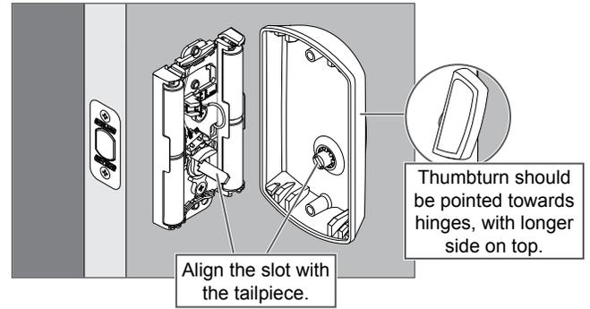
3g Secure the inside cover with two screws.
