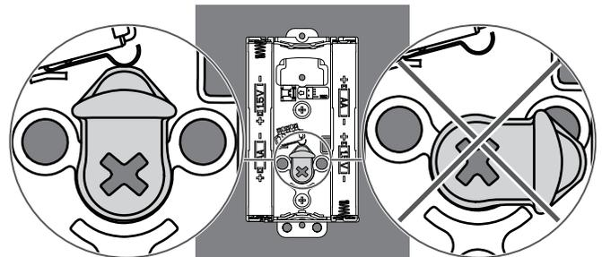
3b Install the inside assembly on the inside of the door.
